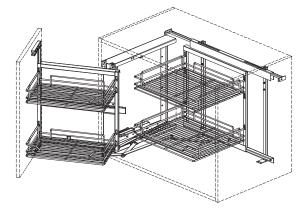
Large basket: 17-15/32" (456 mm) W x 15-1/2" (394 mm) D x 3-11/32 (85 mm) H Small Basket: 17-5/32" (436 mm) W x 10-1/8" (257 mm) D x 3-11/32" (85 mm) H
