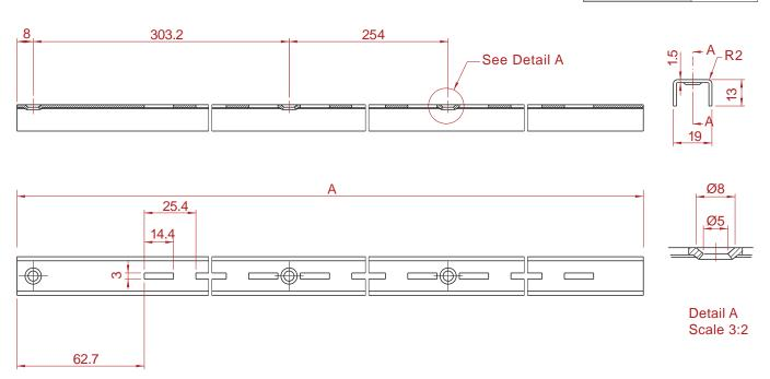
NOTE: Proper installation and mounting required. Tested to meet or exceed ANSI/BHMA performance standards. Weight limits are based on standards mounted on 16" centers utilizing all provided fastener holes. Mounting fasteners must individually provide at least 650 lb tensile pullout and 900 lb sheer strength.
