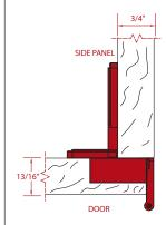
Side Panel 3/4" (19 mm) Door Thickness 3/4" - 13/16" (19–21 mm) Hinge Overlay 3/4" (19 mm) Door Overlay 19/32" (15 mm) 5/32" (4 mm) Reveal Opening Angle 270° Cup Bore Ø 35 mm x 13 mm depth 45 mm Centers x Ø 8 mm Dowels
