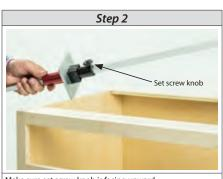
Make sure set screw knob is facing upward. Loosen set screw.
